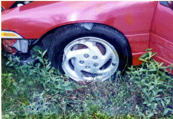
Left front wheel showing rim damage due to high speed impact with curb
