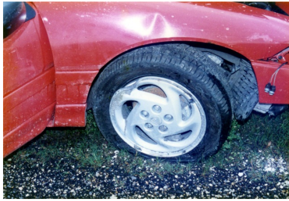
Right front wheel showing rim damage due to high speed impact with curb
